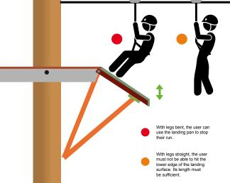
With an articulated joint to reduce strain on the platform and pressure on the trunk.
